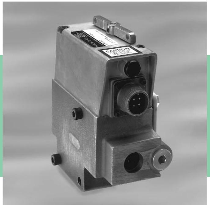
The Moog Controller provides electrical control of the swashplate angle, and so eliminates the need for mechanical interconnection between the operator and the pump. Instead, a simple potentiometer can be located near the operator with a pair of electrical wires running to the Controller. Alternatively, the Controller permits electronic control of the pump-motor combination. Electronic control makes numerous automatic operations possible.
