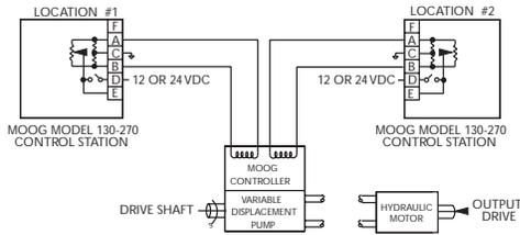
A remote command potentiometer provides the electrical signal for setting the speed of a hydrostatic drive. Moog Snap Trac electronics provide the necessary “black box” to complete the system. Various Snap Trac models are available for industrial use.
