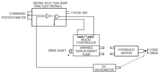
Highest accuracy will be achieved by measuring the output of the hydrostatic drive with an electrical transducer, and using the signal for feedback.
