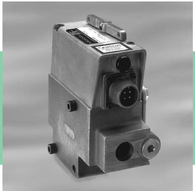
The Moog Controller provides electrical control of the swashplate angle, and so eliminates the need for mechanical interconnection between the operator and the pump. Instead, a simple potentiometer can be located near the operator with a pair of electrical wires running to the Controller. Alternatively, the Controller permits electronic control of the pump-motor combination. Electronic control makes numerous automatic operations possible.
