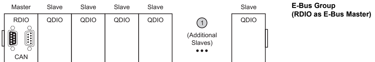
Figure 42: E-Bus Group (RDIO as E-Bus Master)
