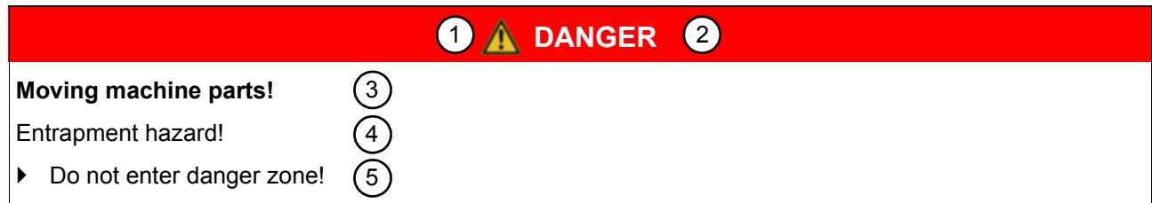
Figure 1: Structure of a warning notice
