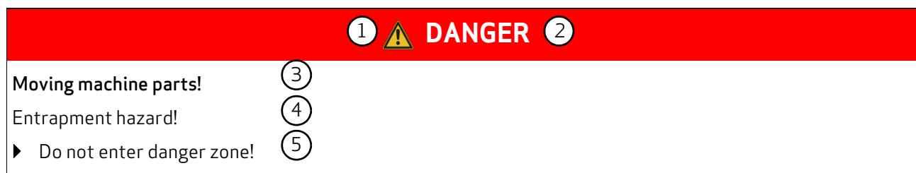
Figure 1: Structure of a warning notice
