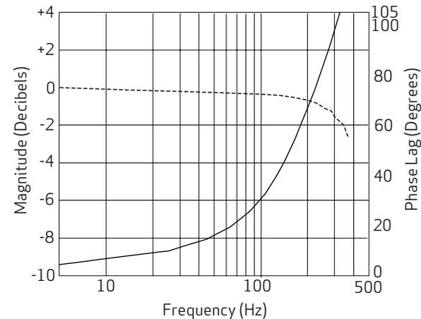
Measured with 40 % signal amplitude, at 3,000 psi (210 bar) pilot or operating pressure, fluid viscosity of 24 cSt, and fluid temperature of 104 °F (40 °C)
