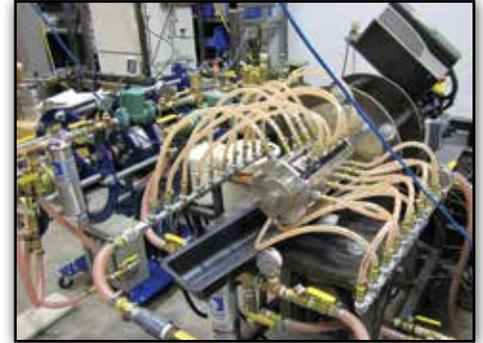
Using a state of the art test facility, various seal recipes are continuously being evaluated. The tests are closely monitored to record even the most miniscule leakage, change in pressure, temperature or torque. This information is helping Moog become an industry leader in fluid rotary union technology.
